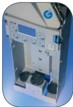
Payout module offers 3 independent & parallel working motors. Pays out up to 6 coins per second. Built-in redundancy in case one motor fails, 4 tubes are still available.
