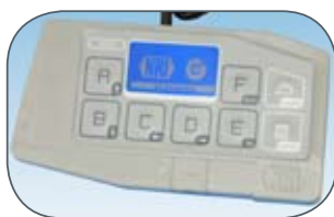
Henri programming module, Operators can download new programs.
